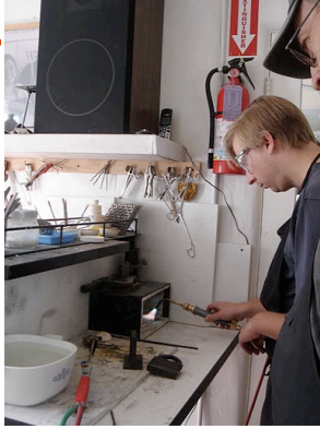
Annealing is needed after milling to soften the metal.
